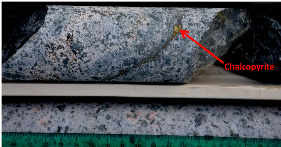
Core photograph, GC04, 167.5-167.6m with Cu @1.48%
